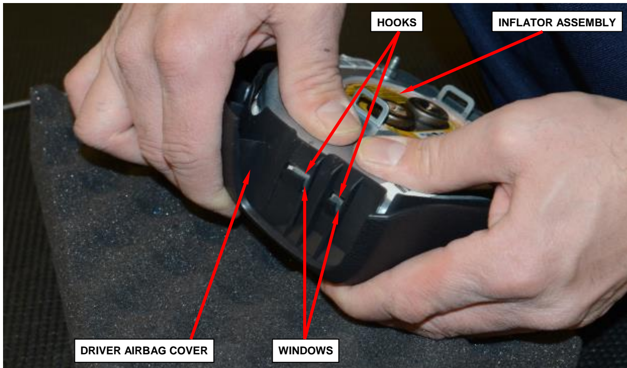
Figure 6 – Left Side Driver Airbag Cover to Inflator Assembly Hooks
